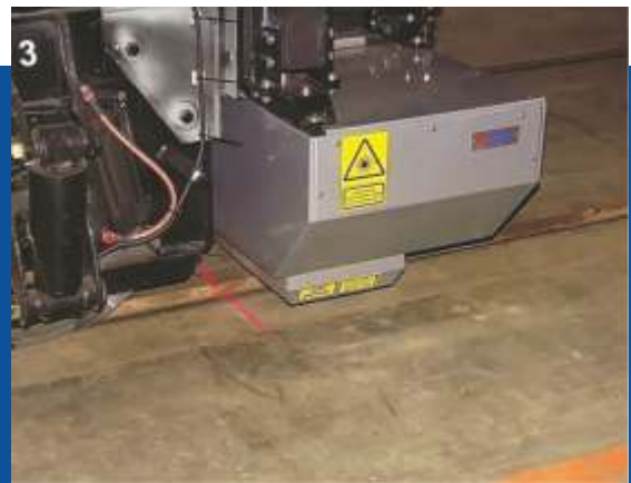
Laser optical measurement module
