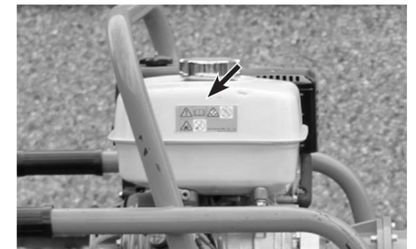
Figure 6: Installation positions for safety signs 4
