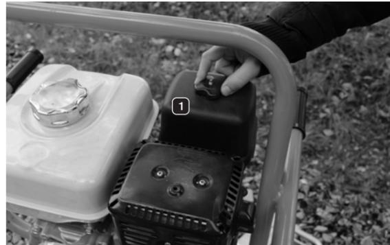
Figure 36: Unscrewing and removing the lock nut
