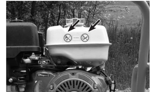
Figure 5: Installation positions for safety signs 3
