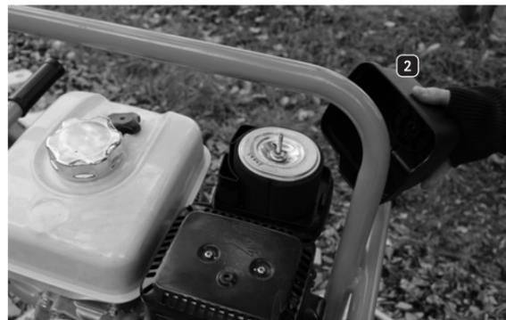
Figure 37: Removing the air filter cover
