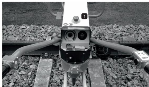
Figure 27: Switching off machine in an emergency
