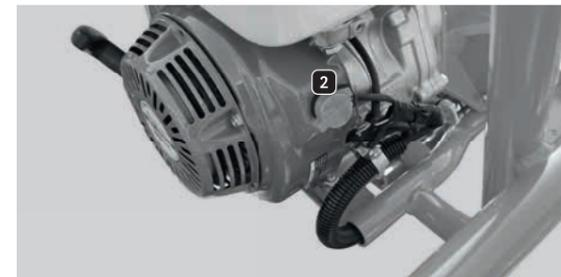
Figure 28: Moving the engine switch to OFF.
