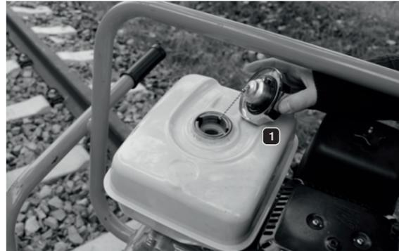
Figure 32: Relevant elements for refueling with fuel
