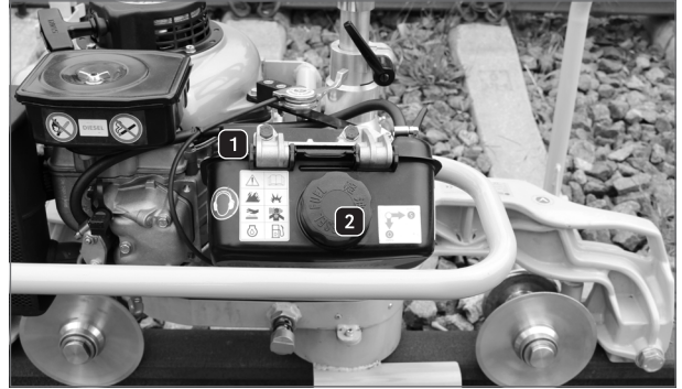
Figure 26: GP 4000 D – Fill in diesel 1
