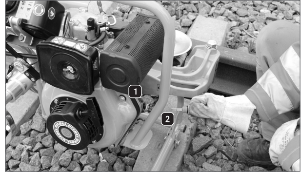
Figure 28: Fill in engine oil – GP 4000 D
