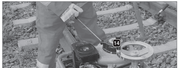
Figure 18: Operating and adjustment controls for diesel engine 1
