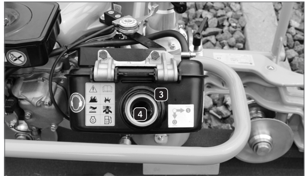
Figure 27: GP 4000 D – Fill in Diesel 2
