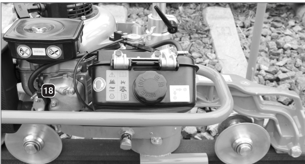
Figure 22: Oil fill plug for cold start
